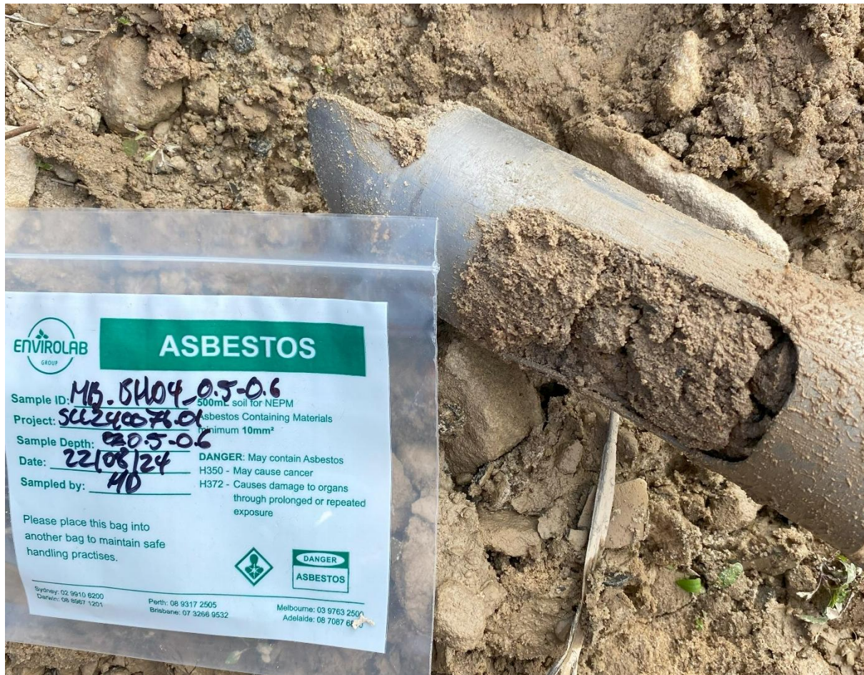
Plate P3. Representative sandy clay material located at BH04.
