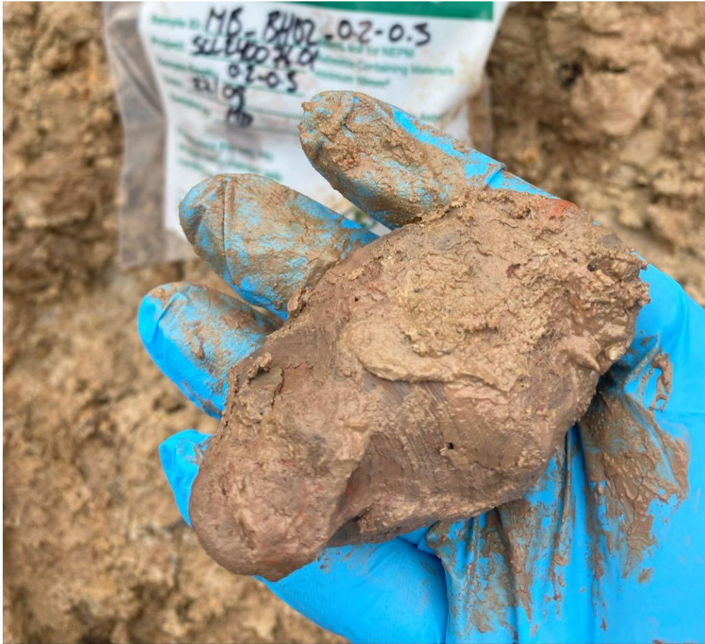
Plate P2. Wet brown/grey clay located within BH02.
